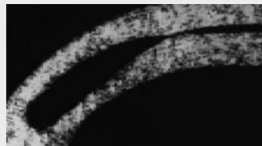
Fig. B.6: Crevice corrosion on a cold strip made from austenitic steel. Sectional view (50-fold enlargement).
